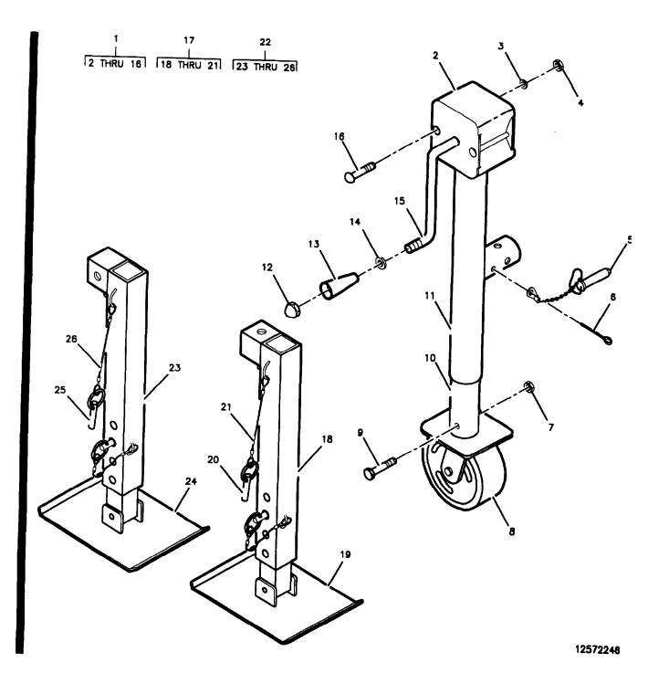
Figure 11. Landing Gear, Leveling Jacks
