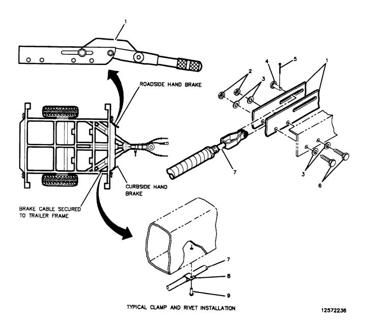
Figure 4. Handbrakes
