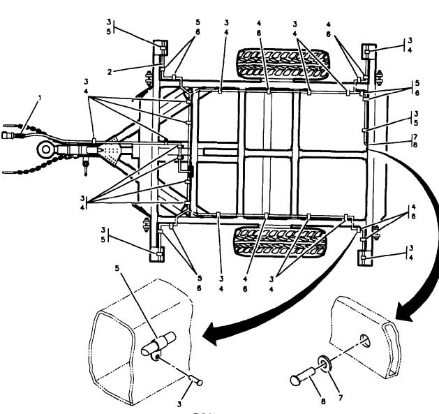
TYPICAL CLAMP AND RIVET INSTALLATION
