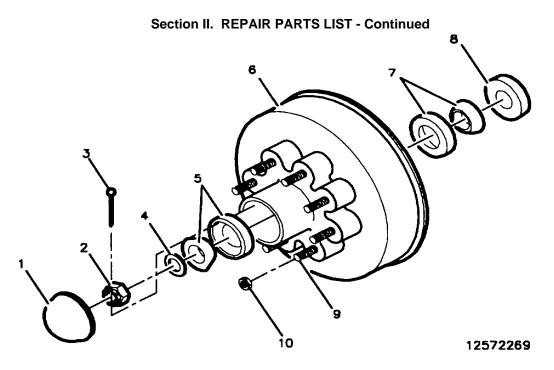
Figure 7. Brake Drum
