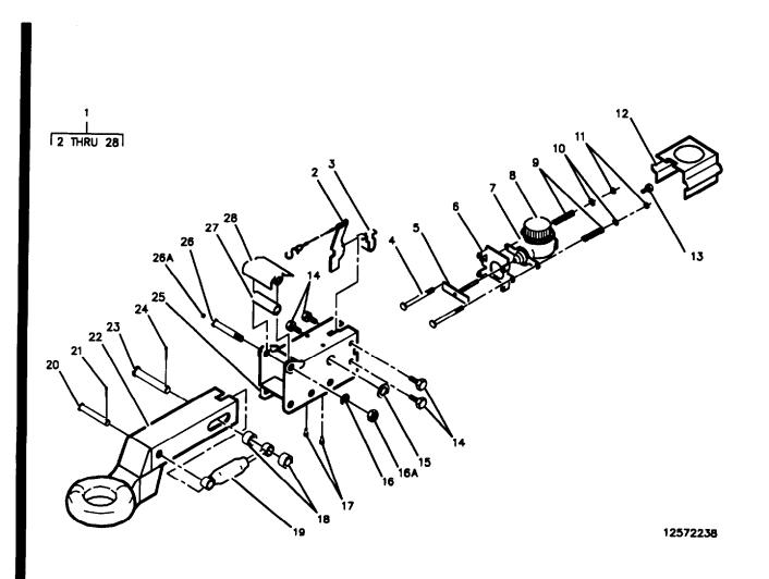
Figure 6. Brake Actuator Assembly (Sheet 1 of 2)
