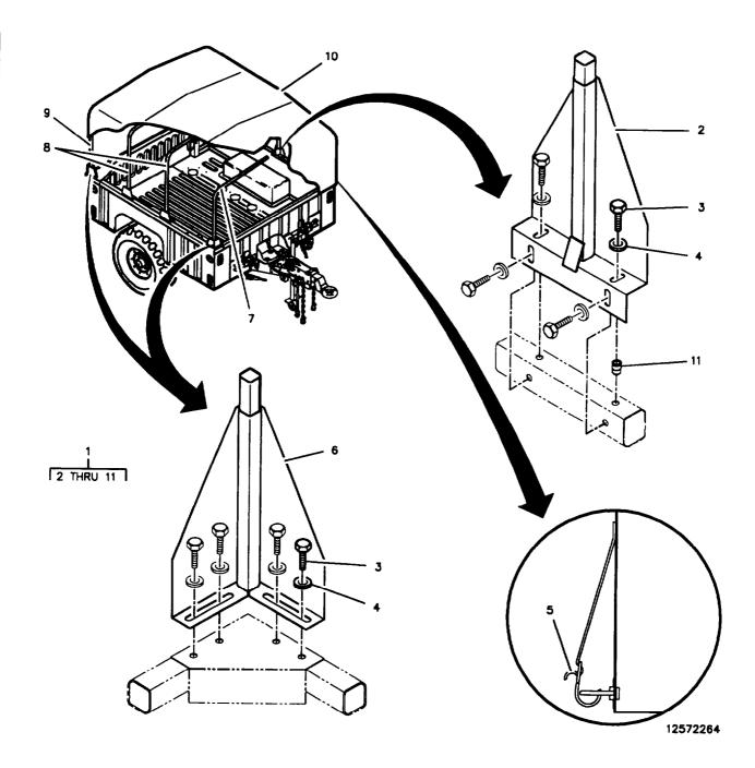
Figure 16. Cargo Body Soft Top Installation Kit
