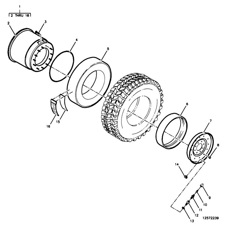
Figure 8. Wheel and Runflat Assembly
