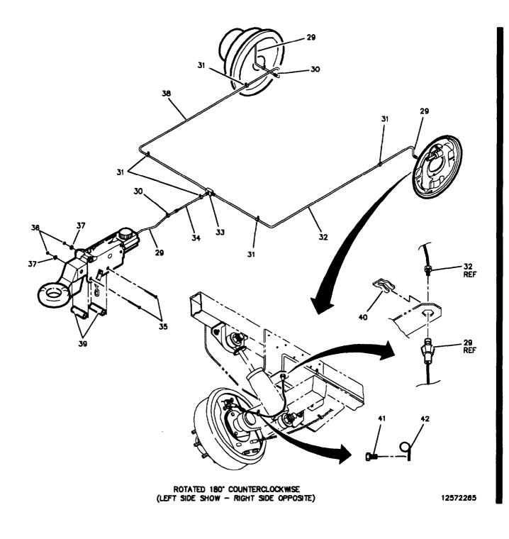
Figure 6. Brake Actuator Assembly (Sheet 2 of 2)
