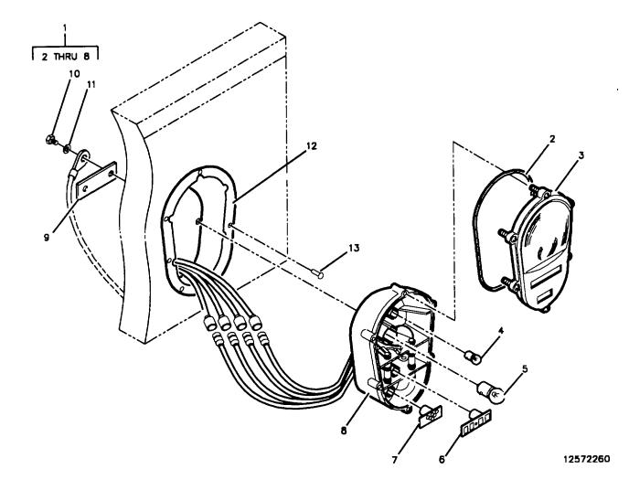
Figure 1. Trailer Lights (Sheet 1 of 2)
